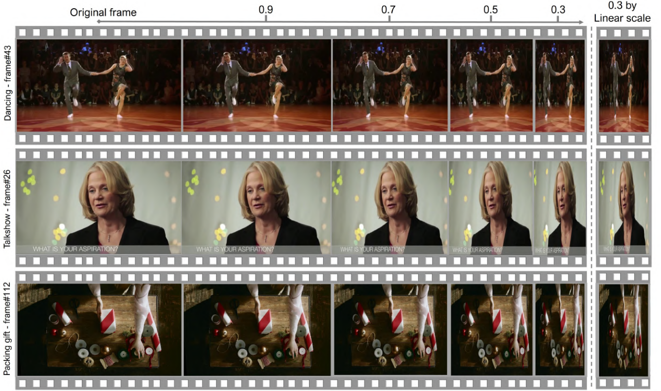
Fig. 4: Performance of our method on different video contents by retargeting to ratio from 0.9 to 0.3 of width.
