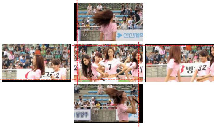
Fig. 6 Clipping window boundary. We identify the rightmost left boundary, the leftmost right boundary, the topmost bottom boundary, and the lowest top boundary of all frames as the boundaries of the clipping window.
